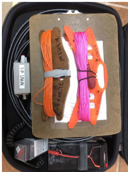
Finally the Unun, Clipboard, Antenna, Counterpoise, Throw Line, Checklist, and the K2 Reference Card
